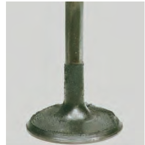
Picture E - Intake valve after P.i. treatment
